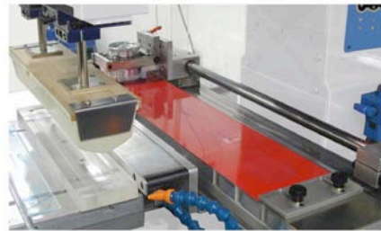
Side way ink cup for long image printing
